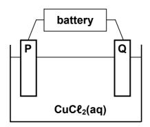
When the cell is functioning, a gas is released at electrode **P**, whilst electrode **Q** is coated with a reddish brown layer.
