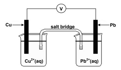
The voltmeter measures an initial reading of 0,3 V.
